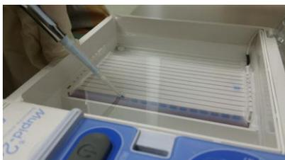
Fig 1: Gel electrophoresis
