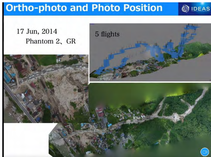
Figure 4 Example of Ortho-photo and photo position renderings from MetaShape
